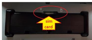
With the iG8 head battery door swung UP, looking into the battery compartment (figure 4 above), the SIM card is inserted with the gold connectors facing UP and the cut-corner is inserted into the hole first (as shown in figure 3.) Push the card into the slot all of the way and it will click into position.
