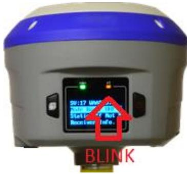
**Note:** you do NOT need the UHF antenna installed if you are using APIS alone. The cellular antenna is under the blue band, just above the metal case.
